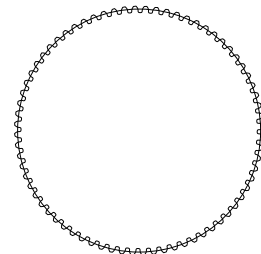
Figure 2.2F, A gear with 72 teeth and a 1-1/2" Pitch Diameter is 48 Pitch.
